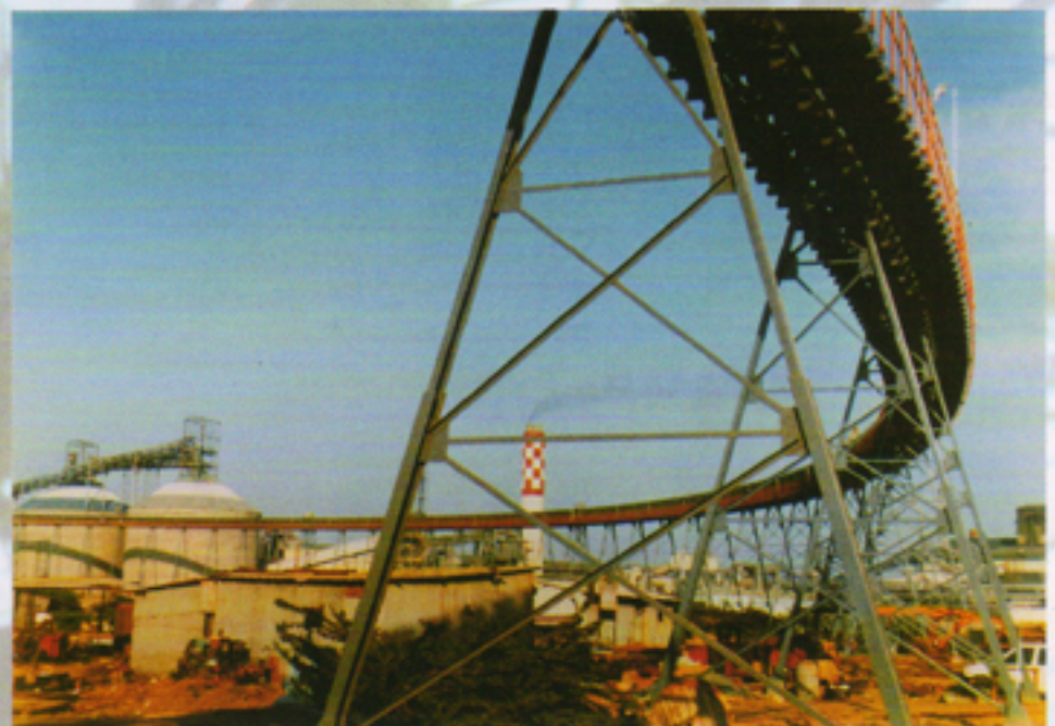
90 degree horizontal curve of Birla Copper Pipe Conveyor
