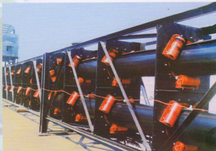
One of the World's Largest Single Flight Pipe Conveyor, length 3.2 Kms. at Birla Copper, Dahej, Gujarat with max. capacity 1760 TPH for carrying Copper Concentrate, Rock Phosphate and Coal.
