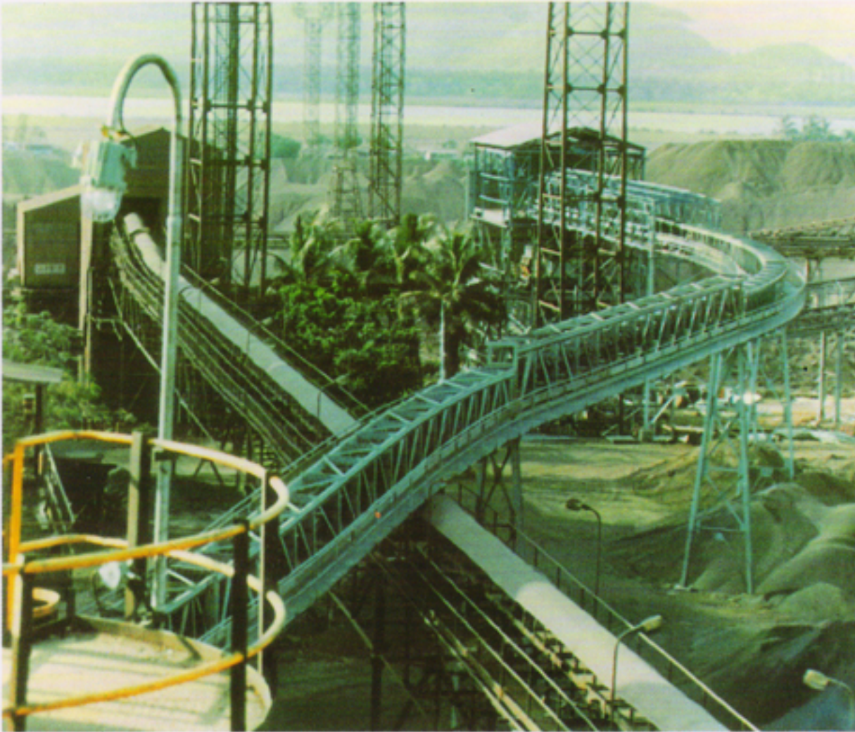
'S' shaped Pipe Conveyor for Vikram Ispat - Revadanda. Length - 180 mts with 400 TPH capacity for Transferring for conveying DRI
